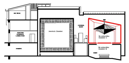
Figure 4.1: Acoutic Testing Service, The red lines show chambers used in measurements
