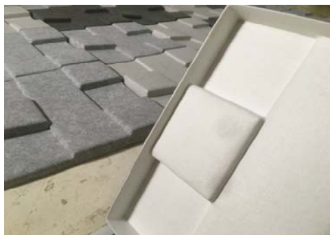
Figure 3: Showing tile cavity
