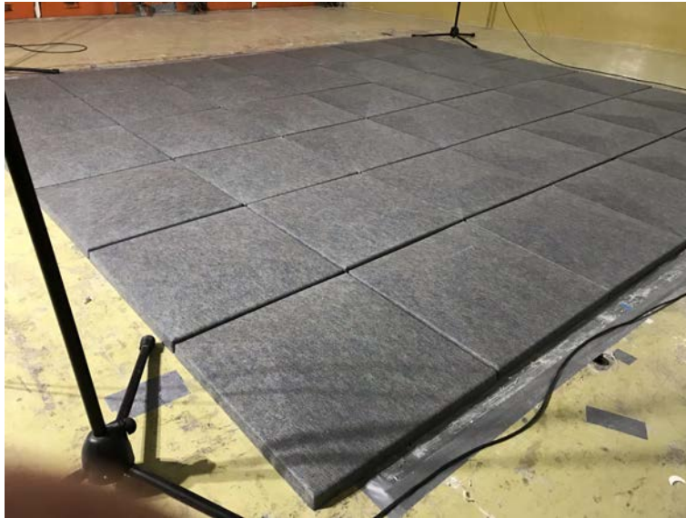
Figure 1.1: Test sample on chamber floor
